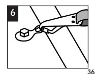
With knee still in child restraint, attach hook to anchor in vehicle. Push down firmly and tighten top anchorage strap.
